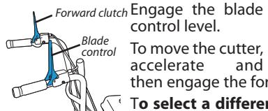
To move the cutter, accelerate and then engage the forward clutch.
