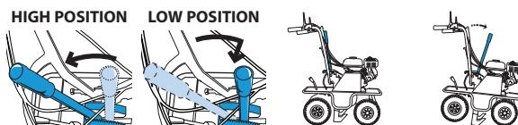
**Engage the blade clutch** only after having carried out the machine switch-on and gear engagement operations.
