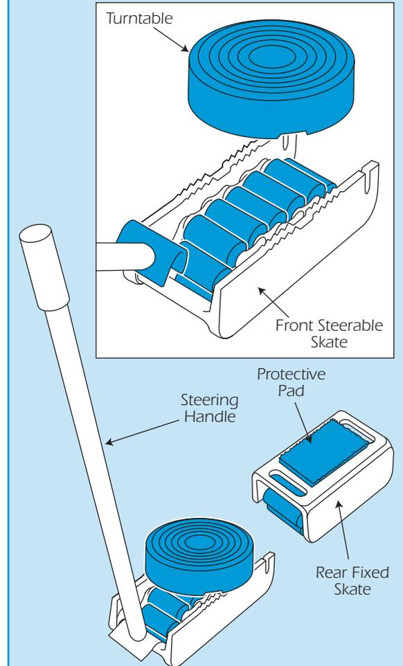
Lower the load onto the skates and double check that everything is OK, make sure that the contact point between the load and skate is strong enough.
