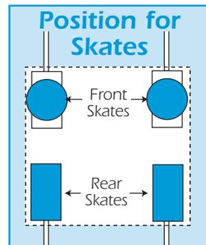
Determine the best position for the two rear skates. Raise the load using suitable jacks then place the rear skates (or pre-locked turntable skates) in position, ensuring that the protective pads are in place.
