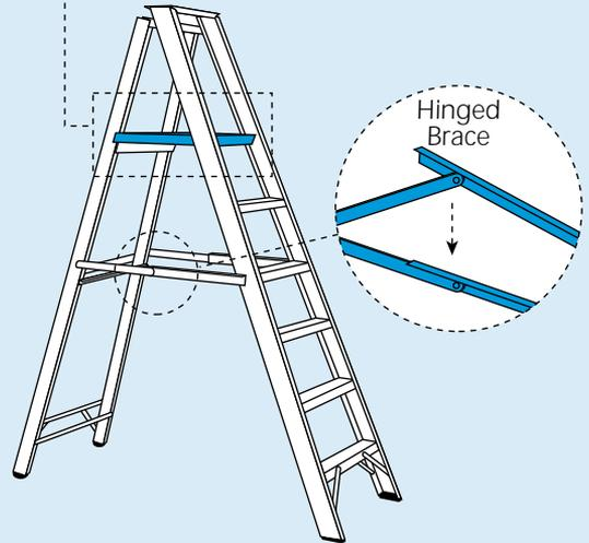
The steps are designed to provide access for light maintenance work. Never use them as a work platform.
